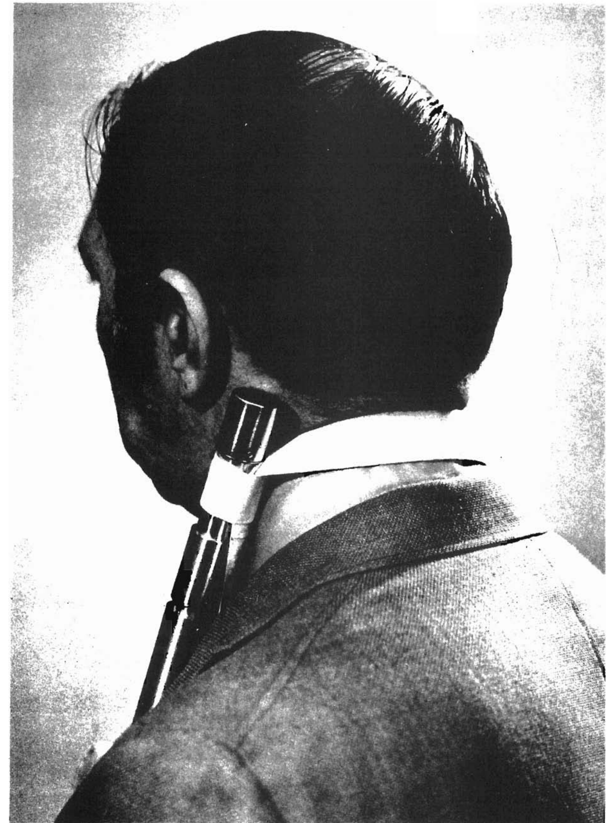
FIGURE B-4 MICROPHONE POSITION RELATIVE TO BLAST OPERATOR'S EAR FOR INSIDE HELMET MEASUREMENT
