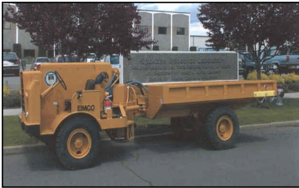
Zero emission utility solution (ZEUS) vehicle, an internal combustion vehicle that operates on hydrogen.
