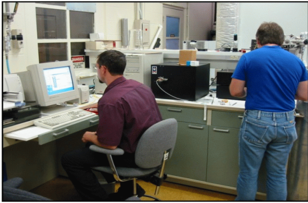
Researchers analyze workplace samples for diesel exhaust particulate using NIOSH Method 5040 for Diesel Exhaust (Elemental Carbon).
