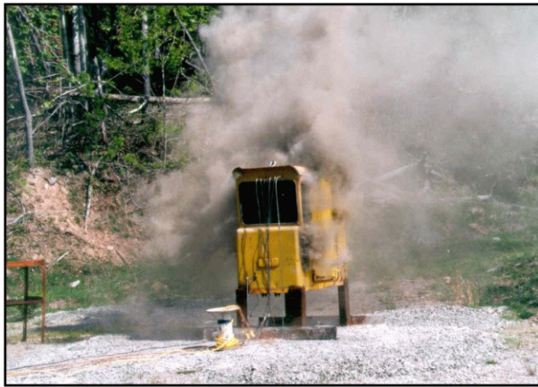
Fire test of noise control materials in a mining vehicle cab.
