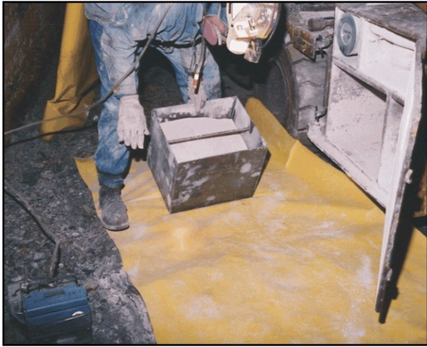
Emptying a dust collector box on a roof bolter.
