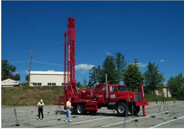
Controlled free-field noise measurements on an air-rotary drilling rig.
