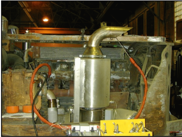
Diesel exhaust upstream and downstream of a particulate matter filter is sampled to determine filtration efficiency for solid carbon core particles (diesel soot).
