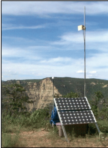
Wireless network connectivity between remote stations of distributed seismic monitoring system.
