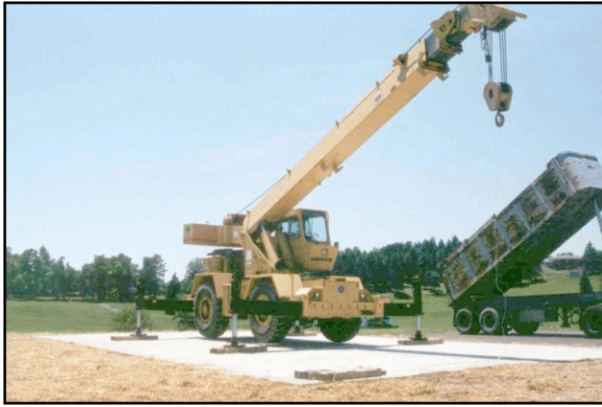
A 22-ton rough-terrain construction crane energized at 4,000 V ac for current measurement tests on a concrete test surface.
