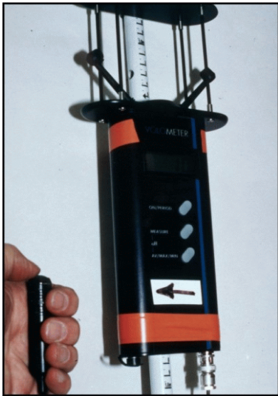
Handheld ultrasonic anemometer capable of measuring very low air velocities.
