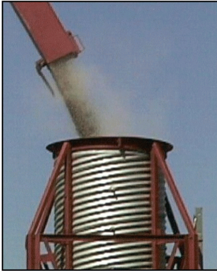
Testing dynamic loads at SRL's scaled ore pass test facility.
