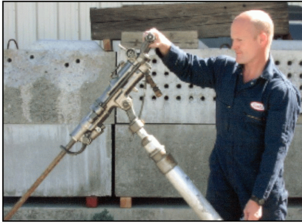
Lightweight jackleg drill—30 pounds lighter than a standard drill steel.
