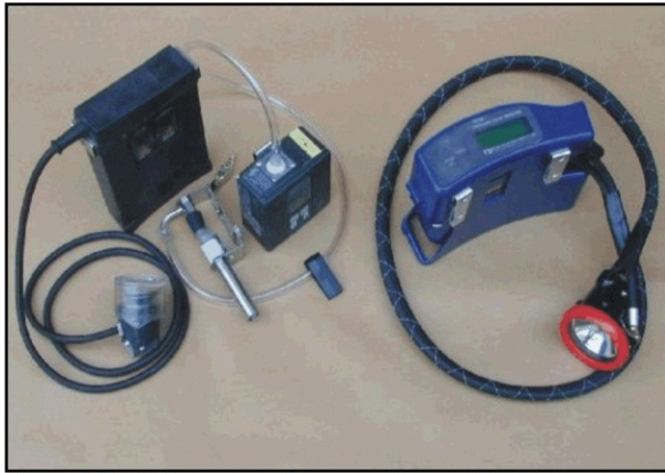
The model of the one-piece personal dust monitor (right) may replace both the cap lamp battery and dust sampling filter (left) for an overall reduction in weight and volume carried by the miner.
