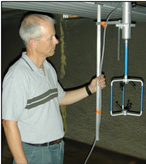
Sonic anemometer used for measuring airflow direction and velocity.
