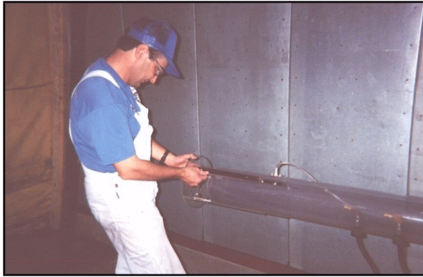
Water-powered scrubber testing to improve air movement and dust capture.
