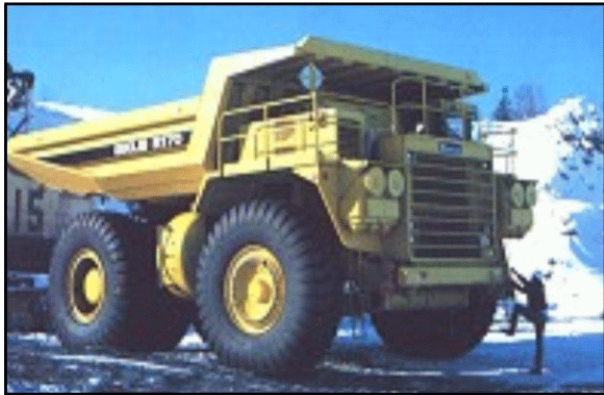
The distance between the first step and the ground can be the most difficult part of equipment access.
