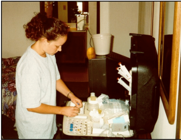
Filter samples are analyzed for lead using field-portable anodic stripping voltammetry.
