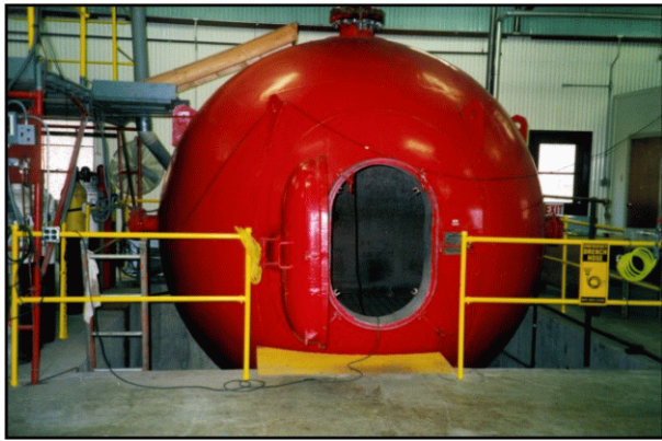
Blasting agent fumes studies are done in NIOSH's explosion sphere. The fumes produced by 1-pound explosive charges are confined in the sphere pending sampling and analysis.
