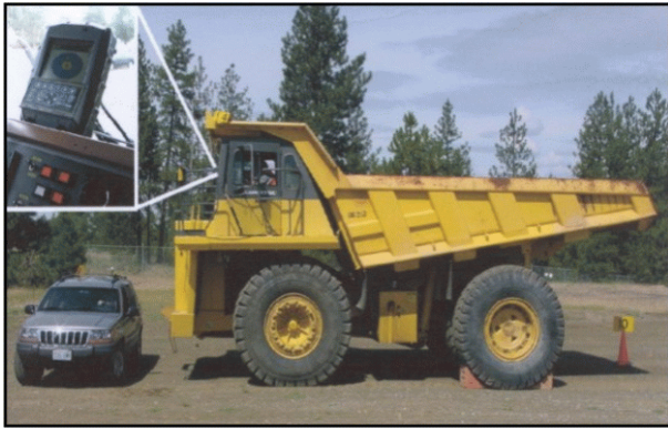
Tests of a GPS-based collision warning system for dump trucks and light vehicles (inlay: truck operation interface).
