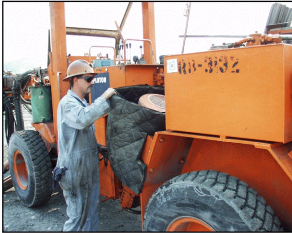
A mechanic removes sound absorption material from a motor to prepare for a noise measurement with an uncontrolled source.
