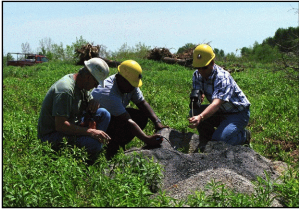
Gas samples are taken from a borehole near a blasting site.
