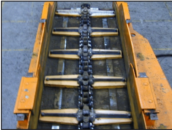
Coated flight bars on the continuous miner's conveyor system.
