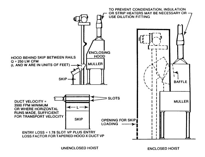
FIGURE IV-8. Skip hoist ventilation for mixers and mullers
