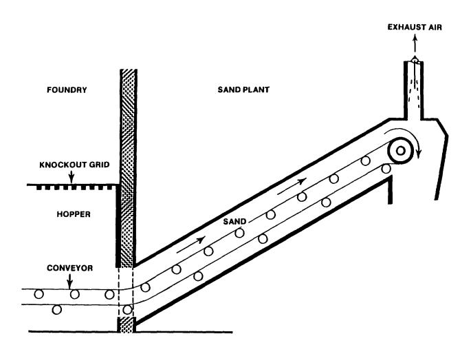
FIGURE IV-4. Local exhaust ventilation on conveyor
