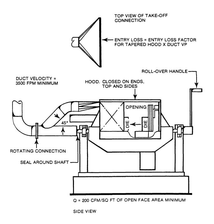
FIGURE IV-10. Small rollover-type coremaking machine
