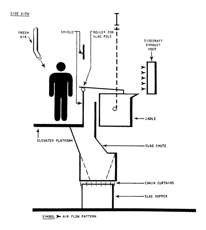
FIGURE IV-13. Slagging station
