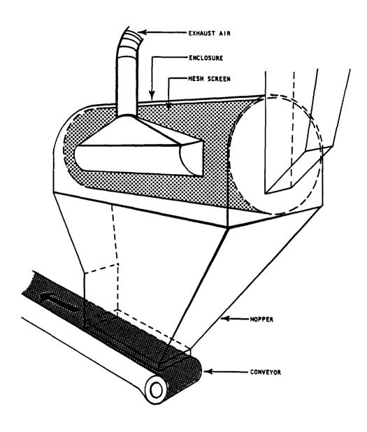
FIGURE IV-6. Local exhaust ventilation at a rotary screen
