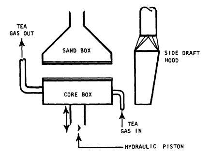
FIGURE IV-12. Cold-box coremaking exhaust
