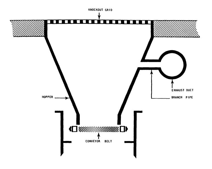
FIGURE IV-3. Local exhaust ventilation below knockout grid
