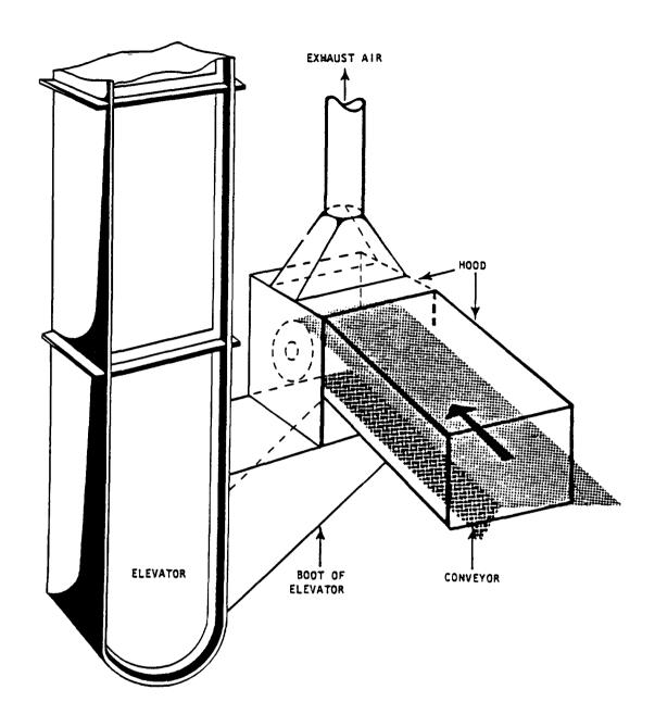
FIGURE IV-5. Hood over transfer point
