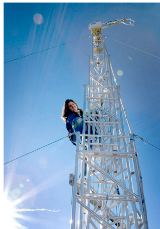
A Los Alamos scientist on an eddy covariance tower used to measure CO 2 flux at the land-atmosphere interface.
