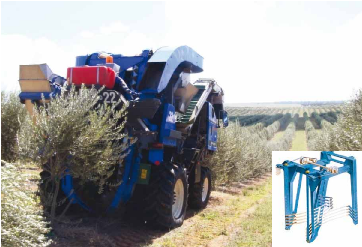
Grape harvester working in 3.5 year-old trees (left) and detail of the picking mechanism (right)
