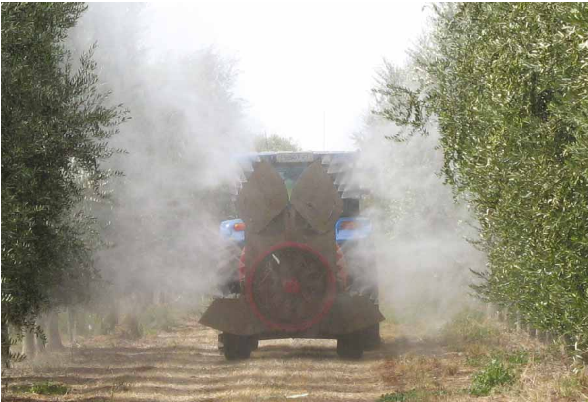
Equipment spraying fruit loosening agents prior to harvest
