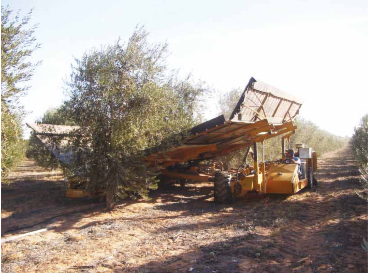
Side-by-side trunk shaker operating in 5 year old trees
