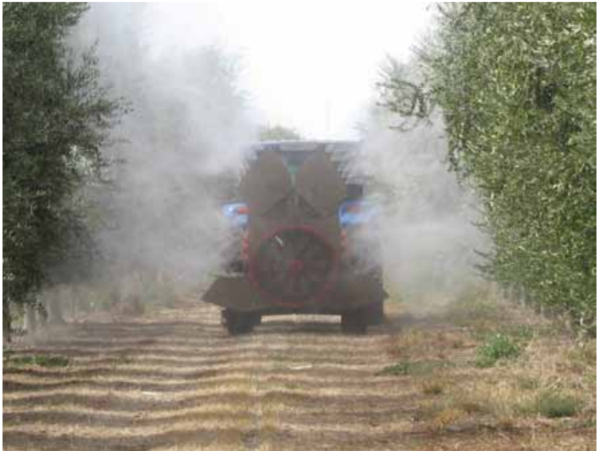
Figure 1. Foliar application of fruit loosening agents by Silvan® sprayer.
