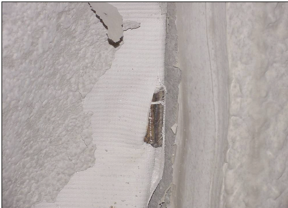
Figure 102.—Initial tear in the woven cloth at the corner steel roof bolt plate position on the inby rib of the X-7 stopping after LLEM test #460, viewed from C-drift.
