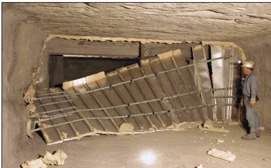
Figure 66.—Debris from steel panel stopping in X-7 after LLEM test #458, viewed from B-drift.
