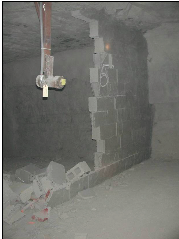
Figure 51.—Part of the inby side of X-6 dry-stacked hollow-core concrete block stopping remaining after LLEM test #433, viewed from C-drift.
