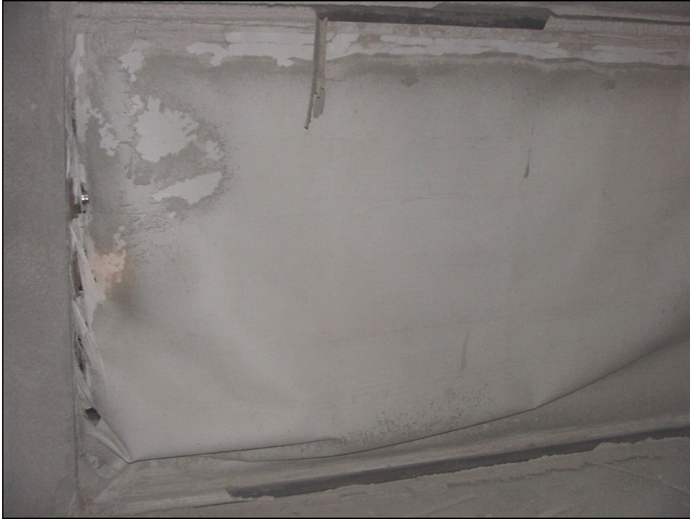
Figure 101.—Tears in the woven cloth on the outby rib of X-6 stopping after LLEM test #460, viewed from C-drift.
