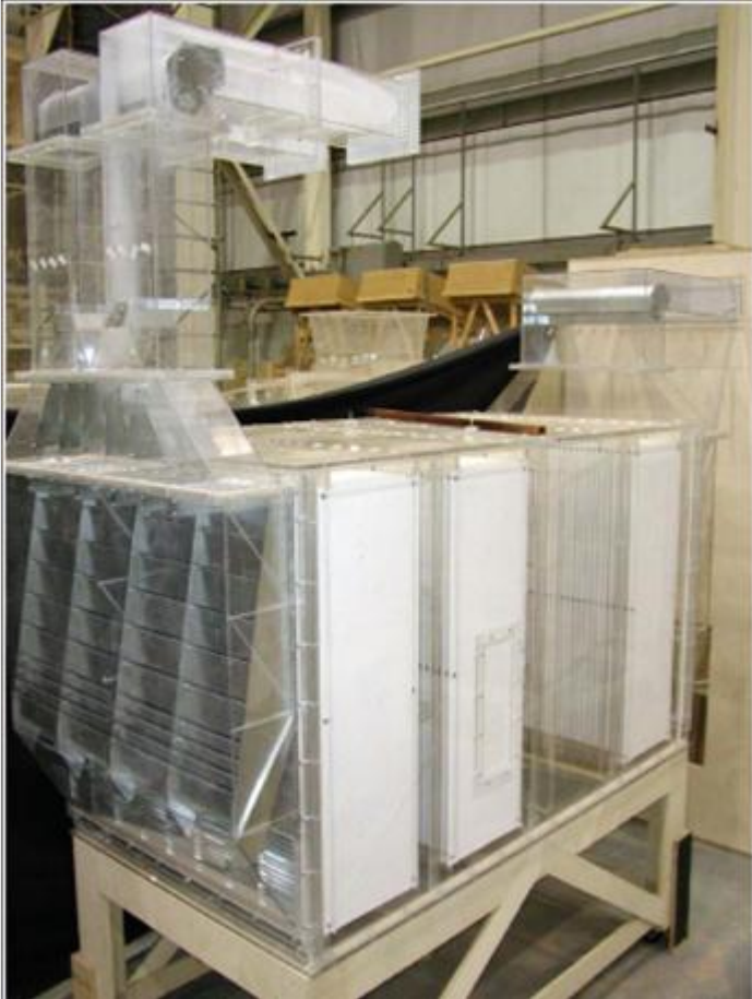
NELS Model 1/2 of 4 ESP boxes on Unit 2 (3 rd field not installed)
