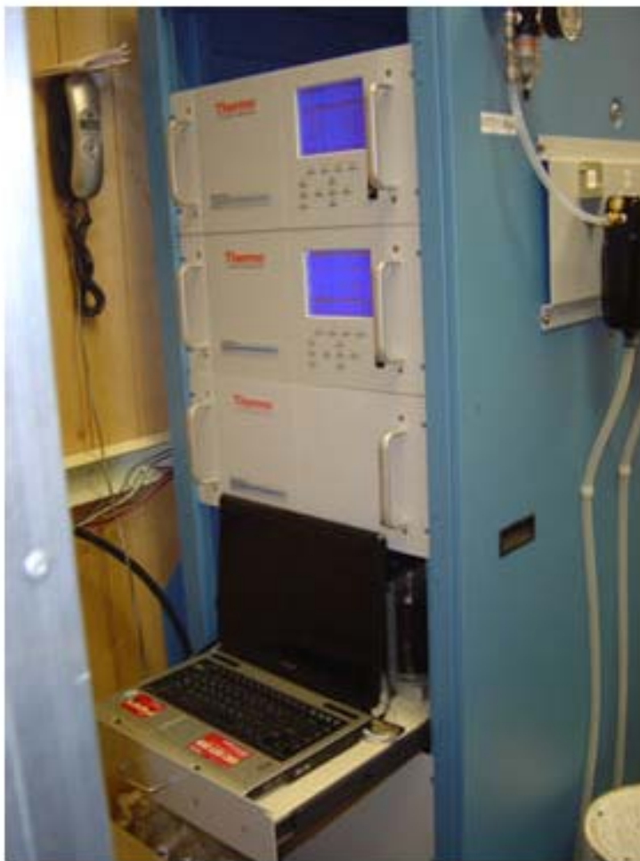
Figure 3-15: Thermo Electron and Tekran CEMs Located in CEM Shelters at Armstrong
