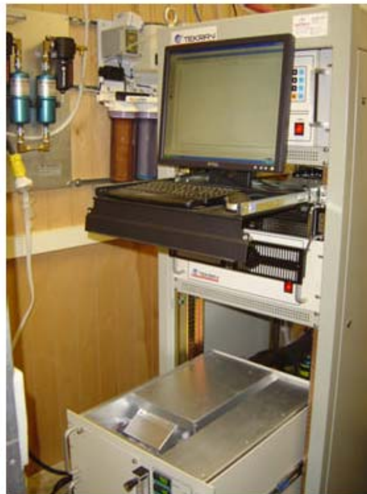
Figure 3-15: Thermo Electron and Tekran CEMs Located in CEM Shelters at Armstrong
