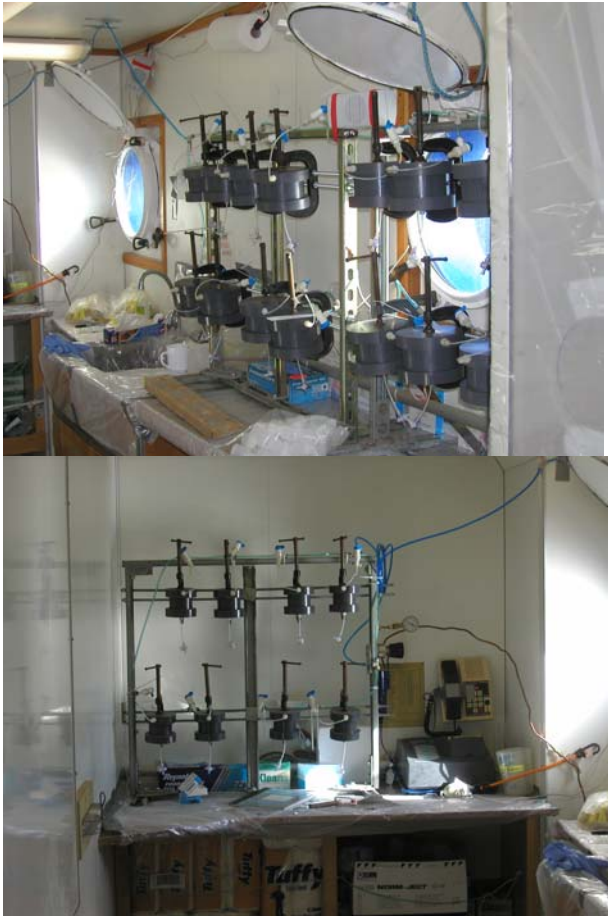
Figure 7: Porewater press lab setup with 24 press ports.
