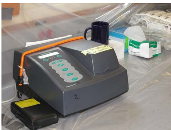
Figure 10: ThermoSpectronic Genesis 20 spectrophotometer used for porewater sulfide analysis.
