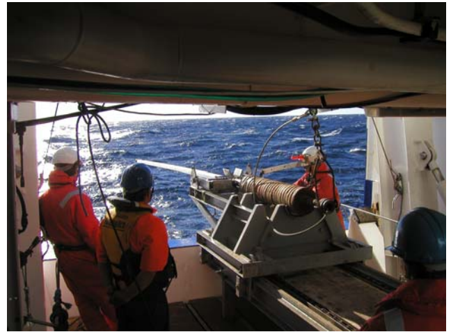
Figure 6: Piston coring system provided by NIWA.
