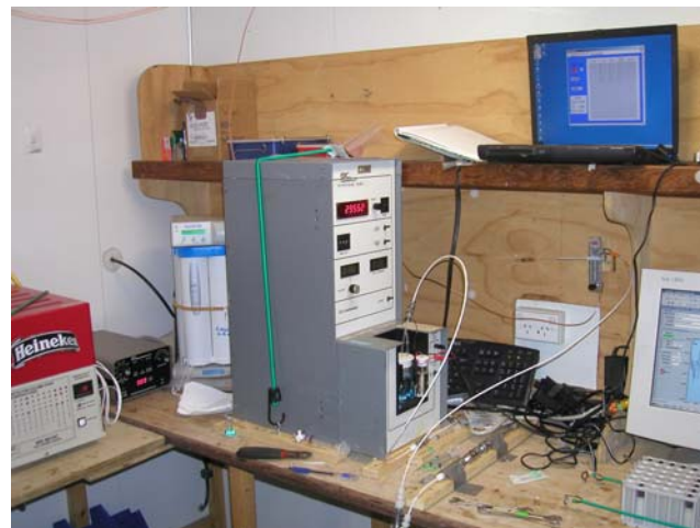
Figure 11: UIC Inc. Coulometric system 030 used for DIC analysis.
