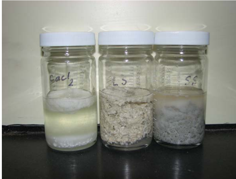
Figure 7.8: Polymer batch test. From left to right: CaCl 2 , limestone and sandstone containers
