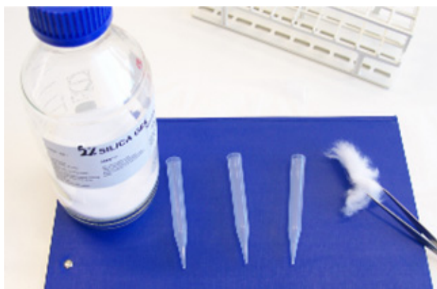
Figure 5.3 Components for “in-house” made columns for separating pigments
