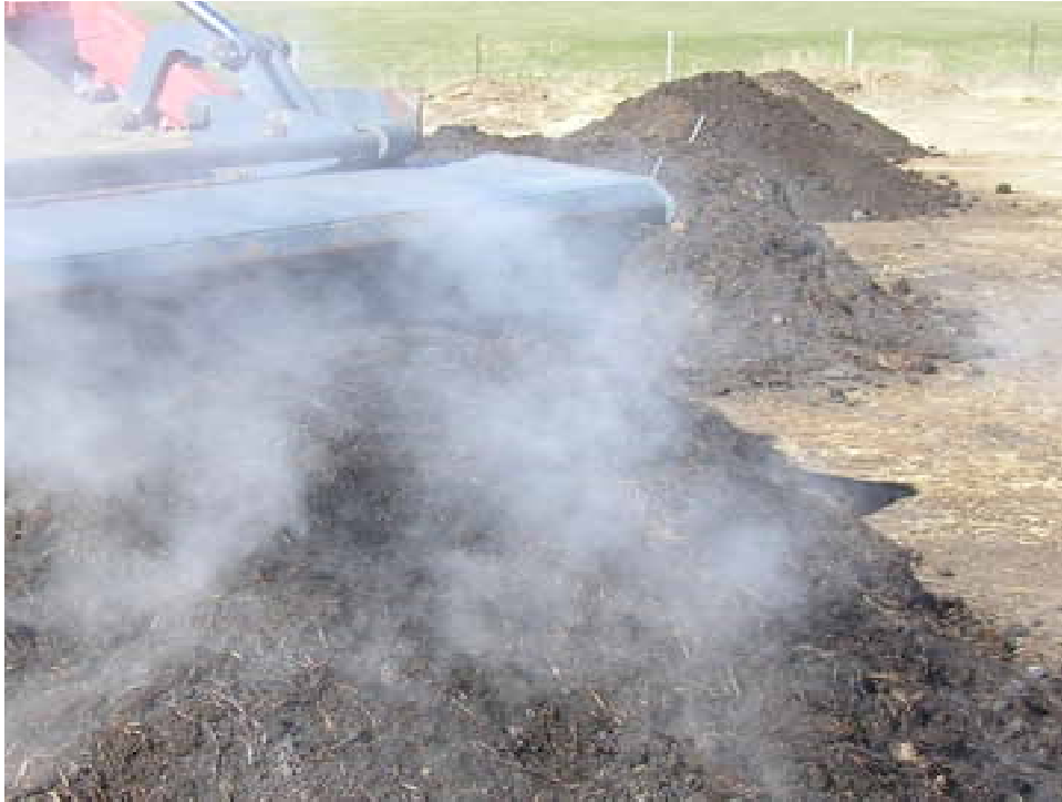
Figure 2 – The lay out of the olive husk trial compost batches. Note the turning operation of the compost heap in the foreground by front end loader, and the steam created in the compost heap by microbial activity.
