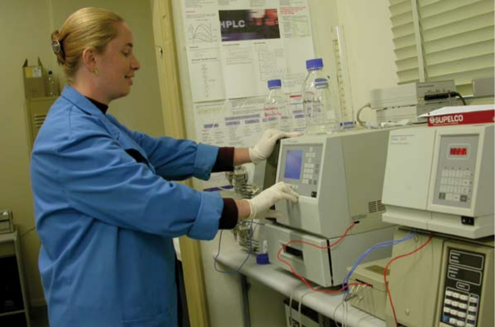
Amanda McFadden, NSW DPI, analyses olive oil by liquid chromatography
