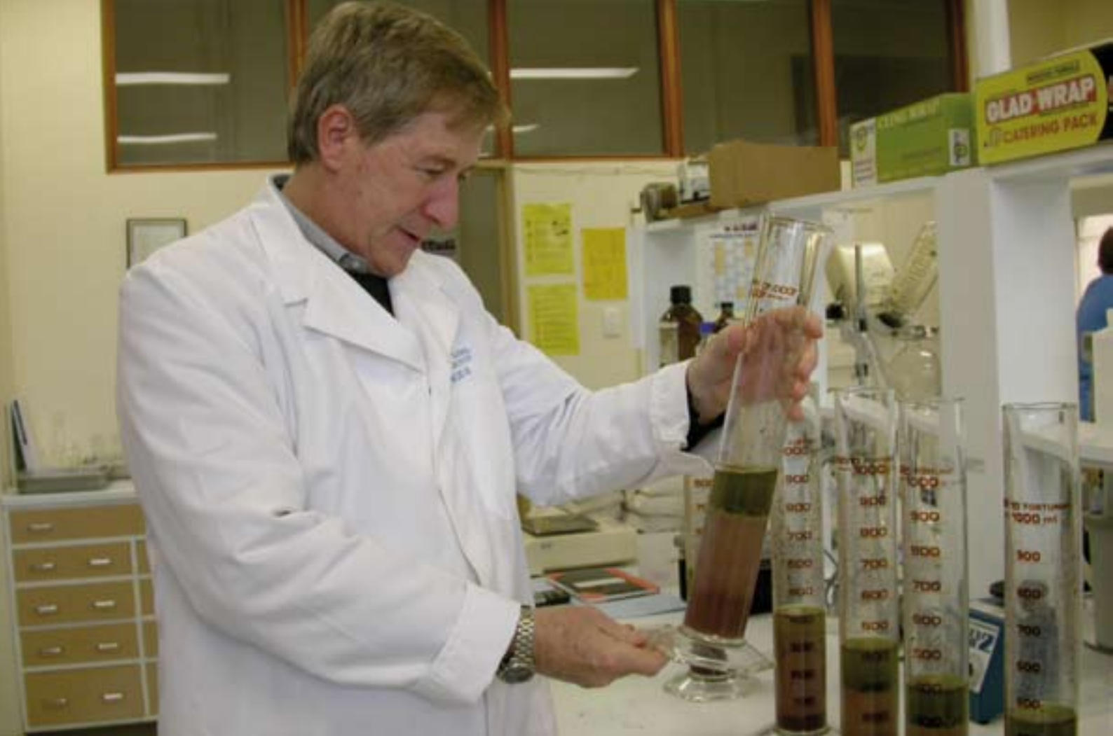
Determining oil content of mechanically extracted olives
