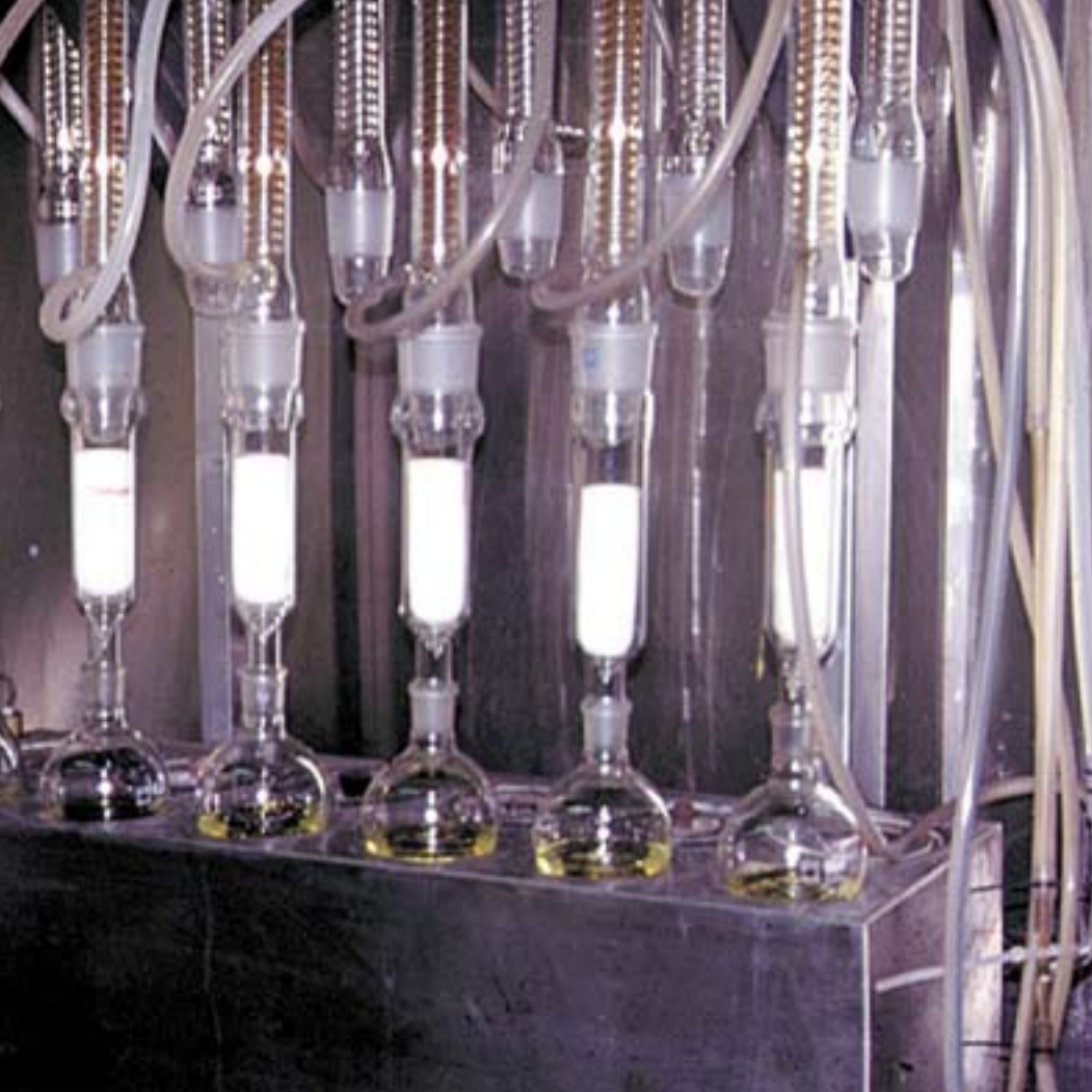
Solvent extraction of olive oil using soxhlet apparatus
