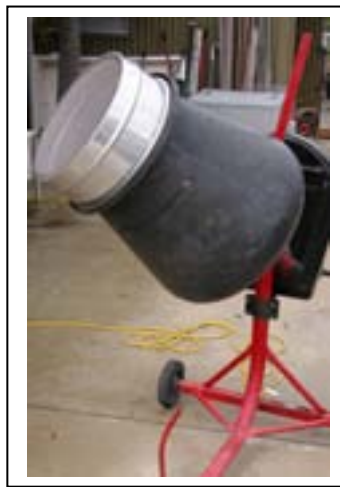
Figure 6 Cement mixer with sieve attachment Figure 7 Sieve 7mm
