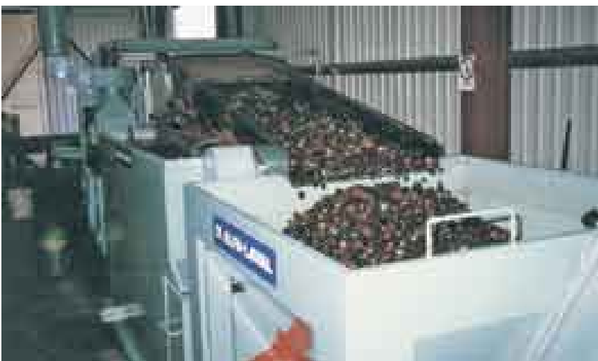
Washing olives on a continuous process system.
