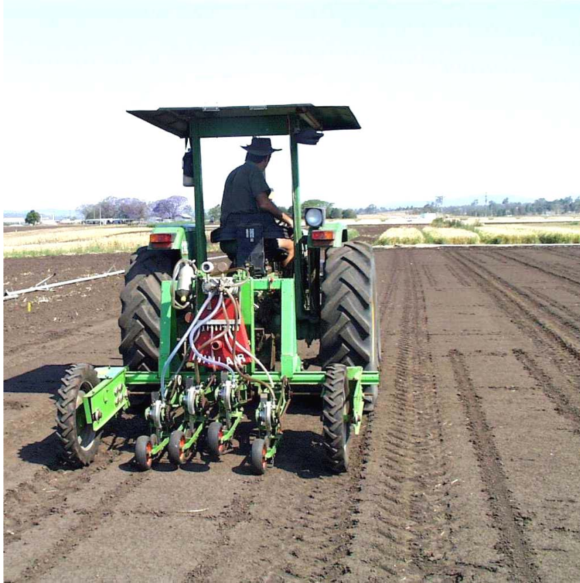
Figure 5.2 Planting of guayule seed using a Mini Air pneumatic planter
