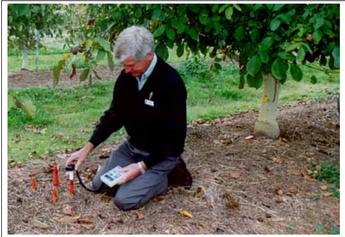
Plate 6. A tensiometer and digital readout used to measure soil water (matric suction).
