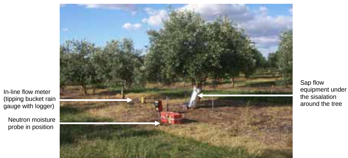
Photo 9 Instrumentation at the Waikerie site
