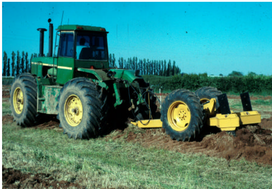
Subsoil on the treelines is modified using a ripper fitted with winged tines
