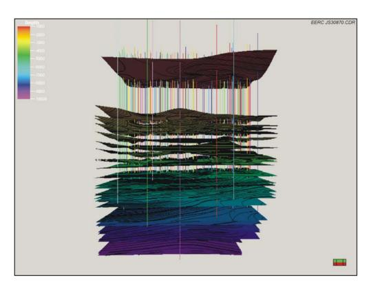
Petrophysical modeling of sealing formations in the Williston Basin based on well log data, geophysical data, and core data from North Dakota Department of Mineral Resources – Oil & Gas Division and commercial data vendors.
