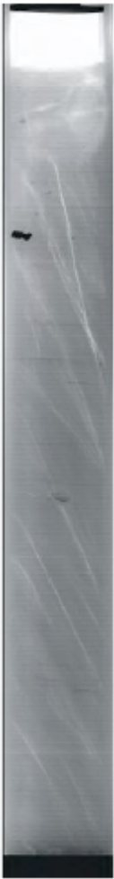
Figure 4: An example longitudinal X-ray image of a one-meter-long pressure core obtained from offshore India containing gas-hydrate bearing fractured clay-dominated sediments. Gas hydrate (lightest shading) occurs primarily as thin, high-angle features filling apparent fractures (photo courtesy of NGHP Expedition 01).
