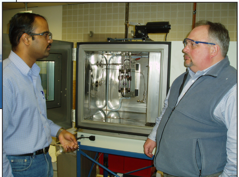
Figure 4. Team members Praveen Singh, a graduate student at the University of Alaska-Fairbanks (UAF), and Pete Stokes, manager of petroleum engineering with Poretchnical Resources of Alaska, discuss hydrate phase behavior apparatus at the UAF Petroleum Development Laboratory.
