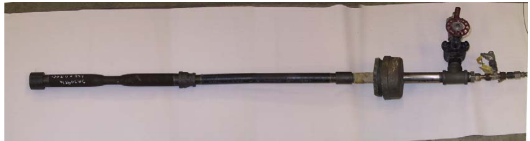
Corrosion/deposition probe assembly
