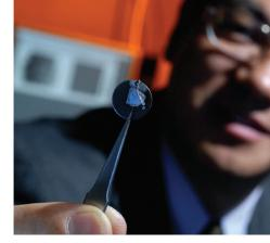
Z.L. Wang, a researcher at Georgia Tech, is using nanowires to generate electricity. Such nanowire systems, assembled on surfaces as small as 2 square centimeters, could some day be used to power implantable medical devices.
