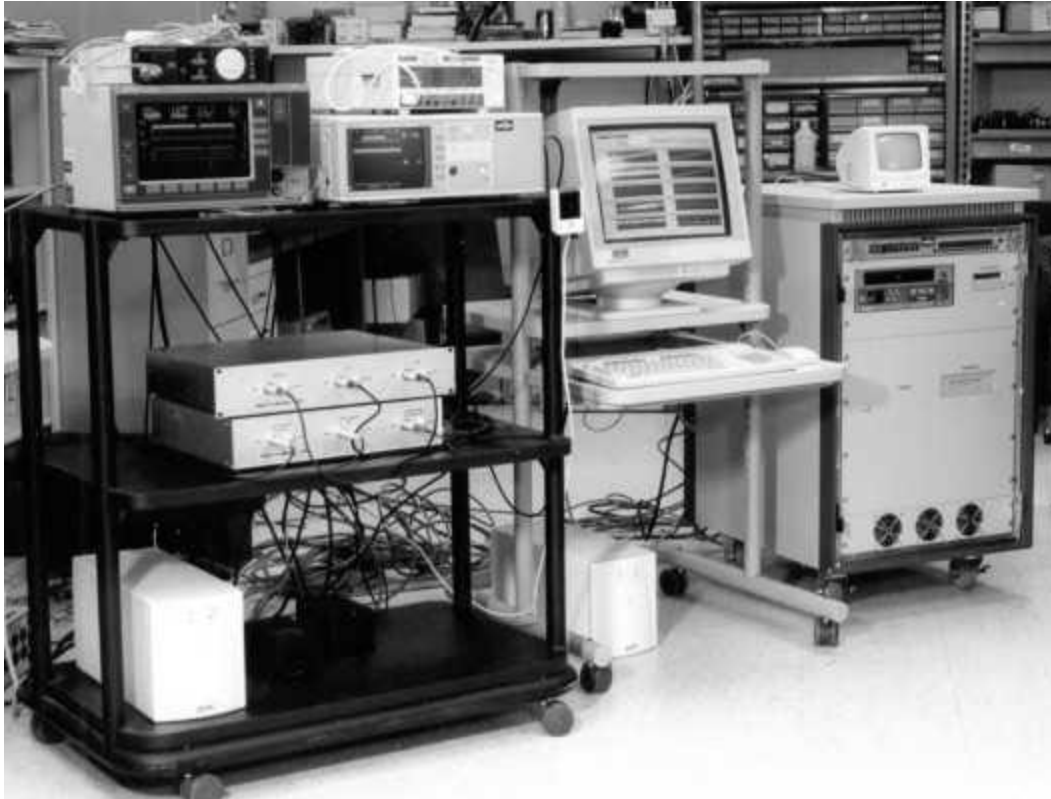
Figure 13. Real-time signal and data acquisition system for recording and displaying high-fidelity physiologic waveforms (signals) from infants in sleep labs
