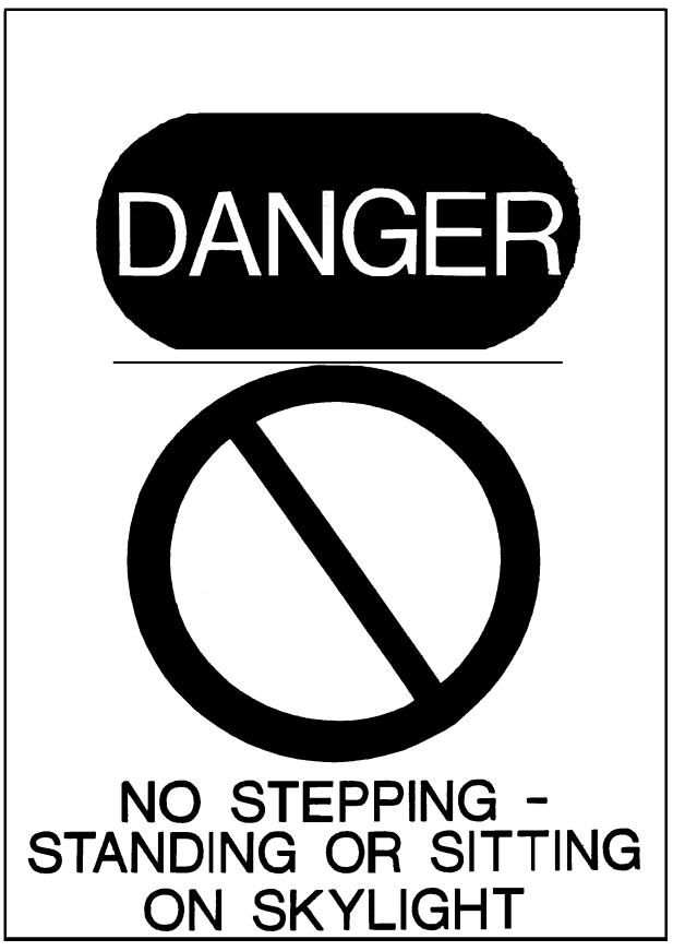
Figure 4. Recommended Accident Prevention Sigh to be Applied to Skylights.
