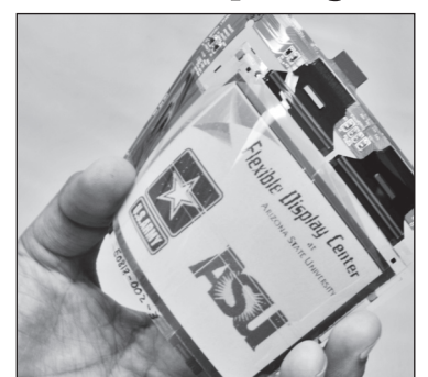
Researchers at ASU's Flexible Display Center have developed a new process for manufacturing high-performance flexible displays on transparent plastic.
