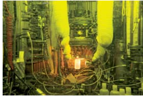
Hot cells at ORNL's Radiochemical Development Center are among the DOE hot cell facilities that may be used to test fuel recycle separations.
