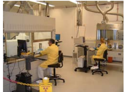
Radiochemistry laboratories provide chemical fume hoods and glove boxes for specialized analyses.
