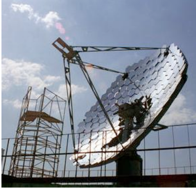
Stirling Dish Solar Generator (Credit: Allan Lewandowski)
