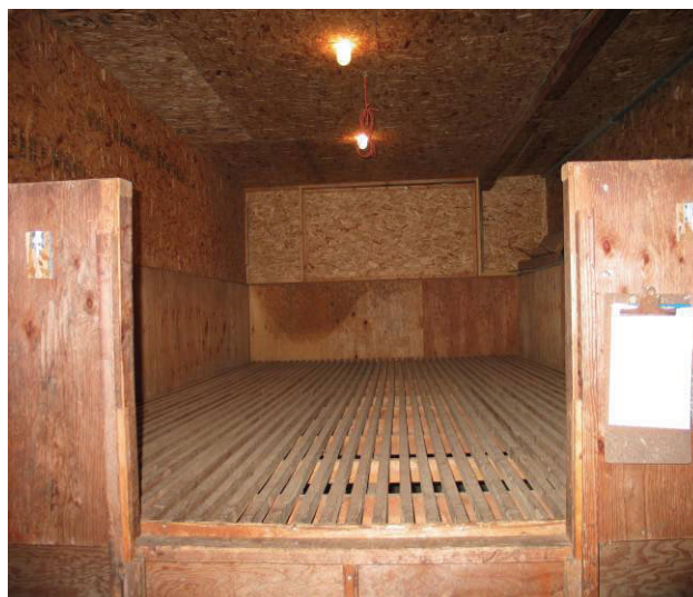
Fig. 2 - Fans force air up through the floor of this homemade seed drying bin.
