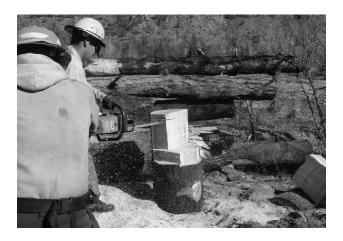
Each student is to bore completely through the cant or stump trying to keep as close to the other flat face as possible (3/8"). If the student cuts completely out, have them try the bore cut again. One stump can be used for this practice by several students.
