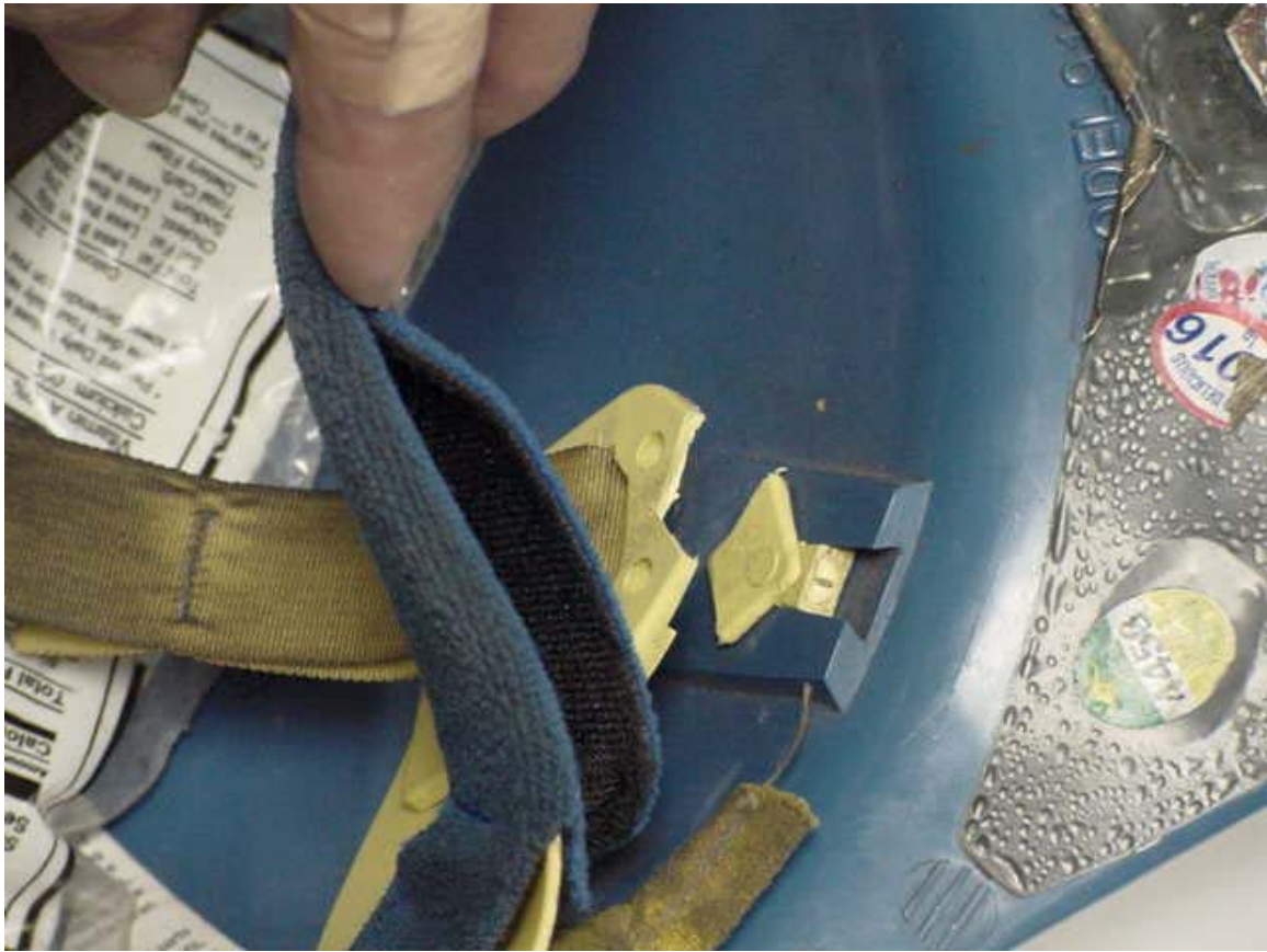
Photo 10 – Helmet worn by victim. Inside of helmet, view of broken headliner strap on left front side. Also, photograph shows the retaining strap band (yellow plastic headband retainer) receded to top of helmet.
