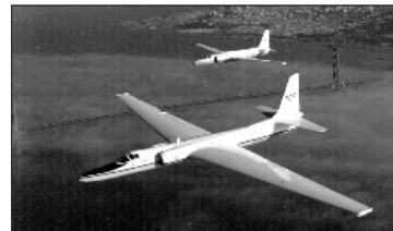
NASA's ER-2 is the country's premier high-altitude civilian research aircraft. Flying in the lower stratosphere, it allows scientists to make in situ measurements for the study of atmospheric chemistry, such as ozone breakdown. It also serves as a testbed for instruments planned for future Earth-orbiting spacecraft.
