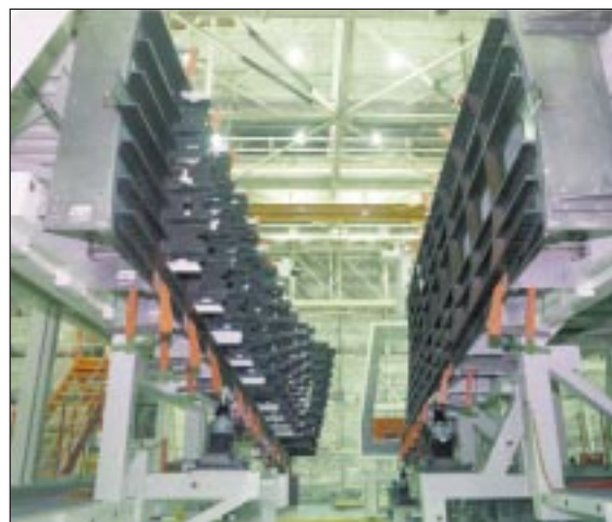
Semi-Span Wing Components Being Installed in the Wing Assembly Fixture
