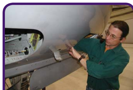
A technician installs a TAMDAR sensor in a Saab 340 commuter airliner at Mesaba Airlines. The Mesaba Airlines fleet will carry the sensors for a year as part of the Great Lakes Fleet Experiment, an operational test of the sensors' ability to provide timely weather forecasts. (Photo: D. Jackson/Mesaba Airlines)
