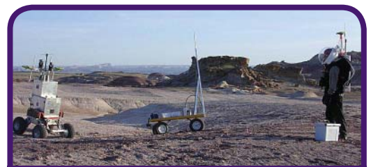
One of the Mobile Agents researchers, dressed in a spacesuit, looks at the computer network relay (center) and a robotic assistant called Boudreaux, which was being teleoperated by a handler. The spacesuits include a communication earpiece and microphone. (Photo: NASA/Mars Society)
