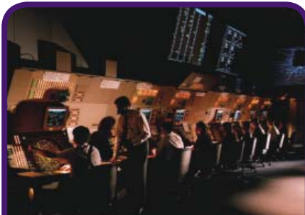
Traffic management advisors sit at consoles at Denver's Terminal Radar Approach Control. Denver and several other center's currently use an older version of the Multi-center Traffic Management Advisor to schedule arrivals and assign runways. (Photo: NASA)
