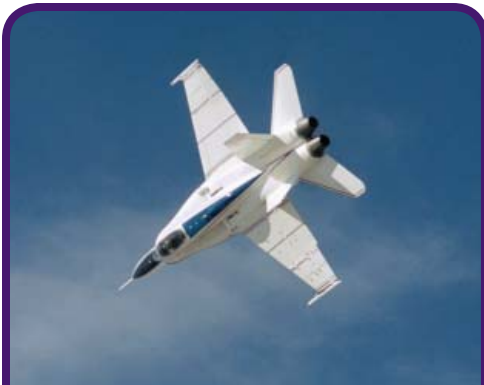
NASA's F/A-18A maneuvers through a test point for the Active Aeroelastic Wing project on December 15, 2004. The stock aircraft was modified with a thinner, more flexible wing skin and structure, new flight control computer software, and a number of sensors that track the wings' flexibility and strain. (Photo: NASA/C. Thomas)
