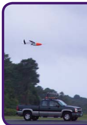
The Aerosonde remote-controlled aircraft is released from its transport truck on the runway at NASA's Wallops Flight Facility, Wallops Island, Virginia. It was sent down the coast to fly through Hurricane Ophelia, a low-energy hurricane. (Photo: NASA)
