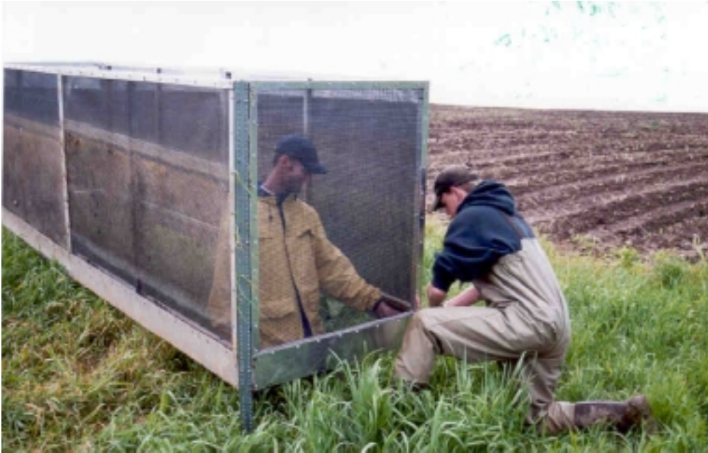
Figure 1. Mesocosm being constructed near an agricultural pond. Note the aluminum frames, as well as the aluminum flashing, and stainless steel stakes extending out from the bottom edge of the enclosure.
