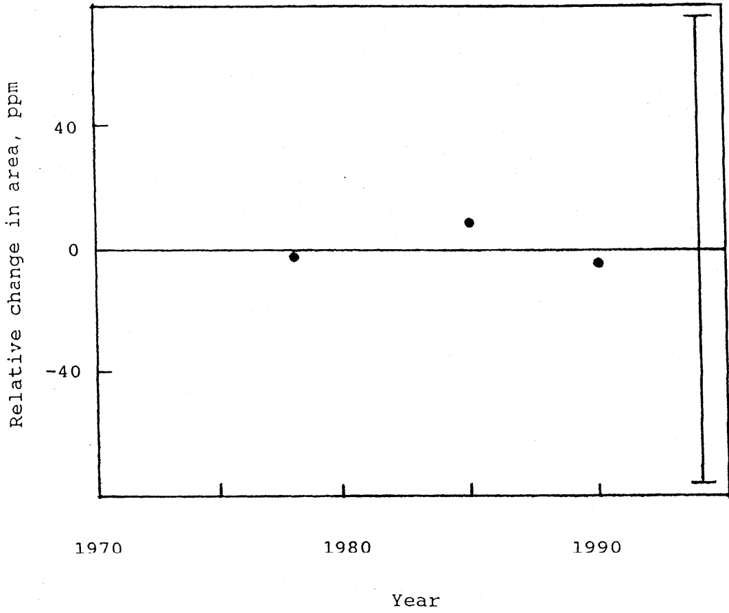
Figure 13. The relative change in the area at the maximum pressure with respect to the average ( 1.679203 \text{ E-}5 ) for PG6 as a function of calendar year. The current total uncertainty is represented by the error bar at the right.
