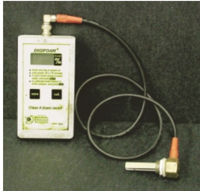
Figure 7—Portable foam concentrate meter.
