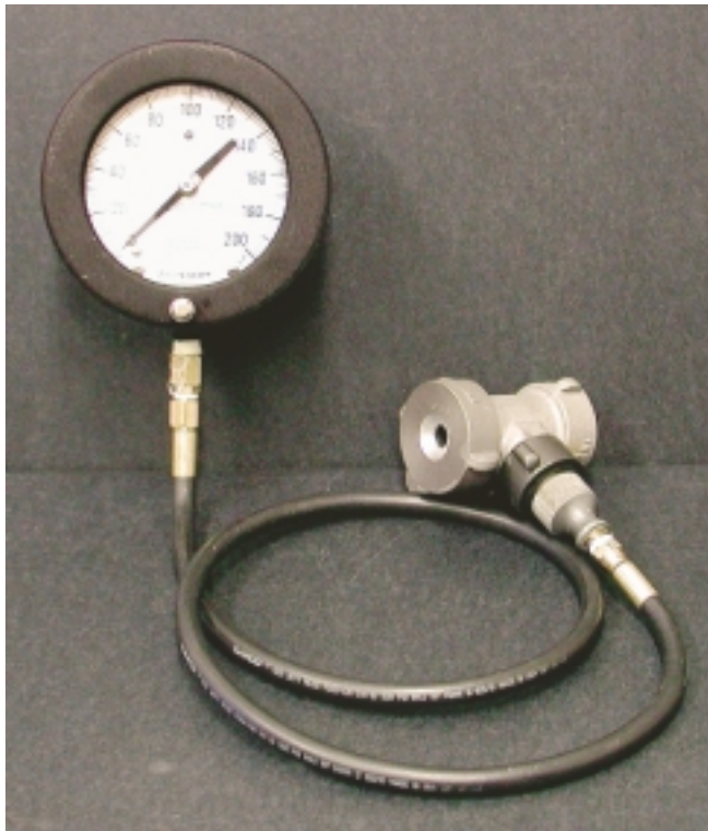
Figure C3 – Photo of square-edged orifice system.
