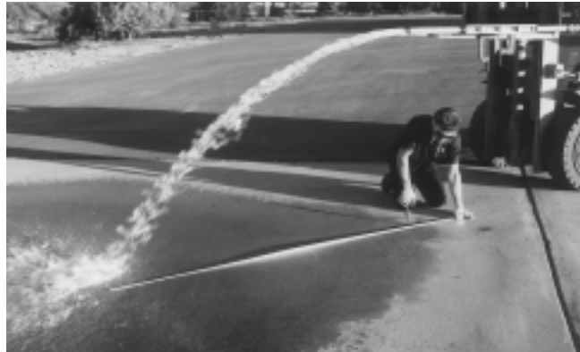
Figure C2—Splash test with 1½ inch pipe at suggested height of 54¼ inches; the calculated flow rate is 84 gal/min.
