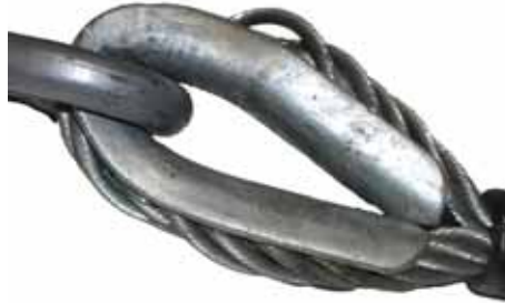
Figure 8. Deformed Thimble and Hook.
