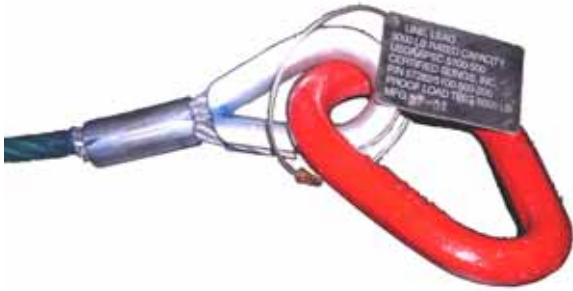
Figure 7. Thimble, Pear Link and Proof Load Tag.
