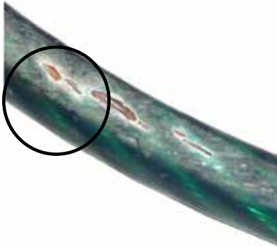
Figure 5. Damaged plastic coated wire rope.
