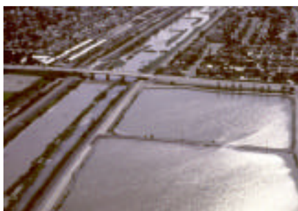
Artificial groundwater recharge in the Santa Ana Riverbed, Orange County Water District, California.
