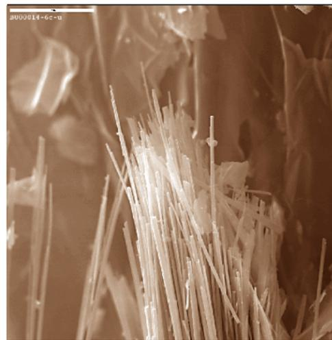
*Scanning electron micrograph of asbestiform amphibole*
