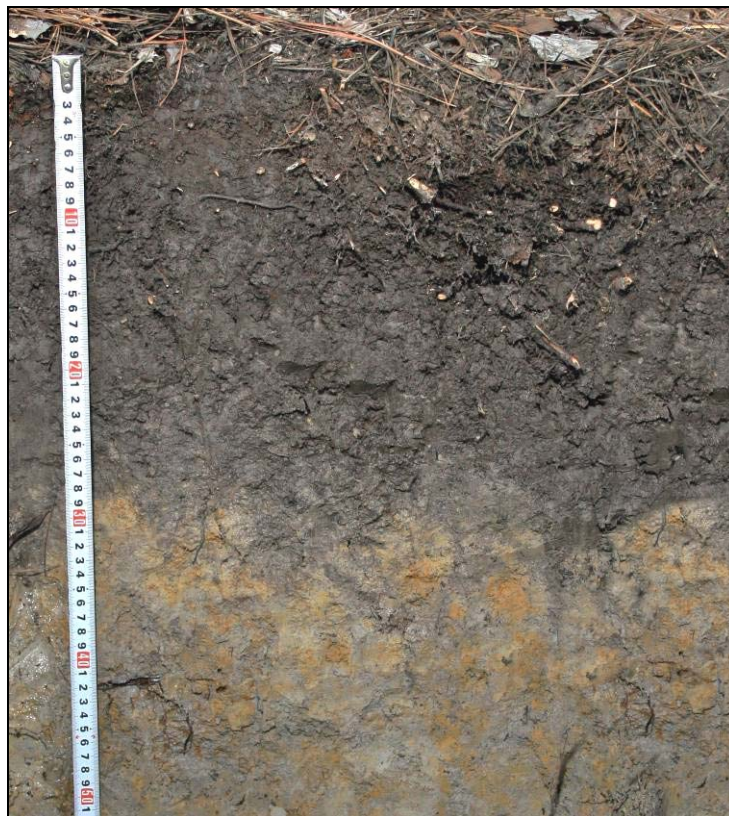
Figure 11. In this soil, a depleted matrix starts immediately below the black surface layer at approximately 11 in. (28 cm).
