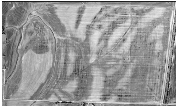
Figure 44. Aerial photograph of an agricultural field with saturated soils indicated by darker colors.
