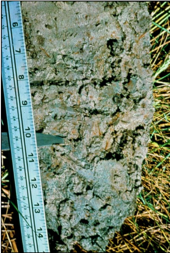
Figure 18. Indicator F3, Depleted Matrix. Redox concentrations are present within a low-chroma matrix.
