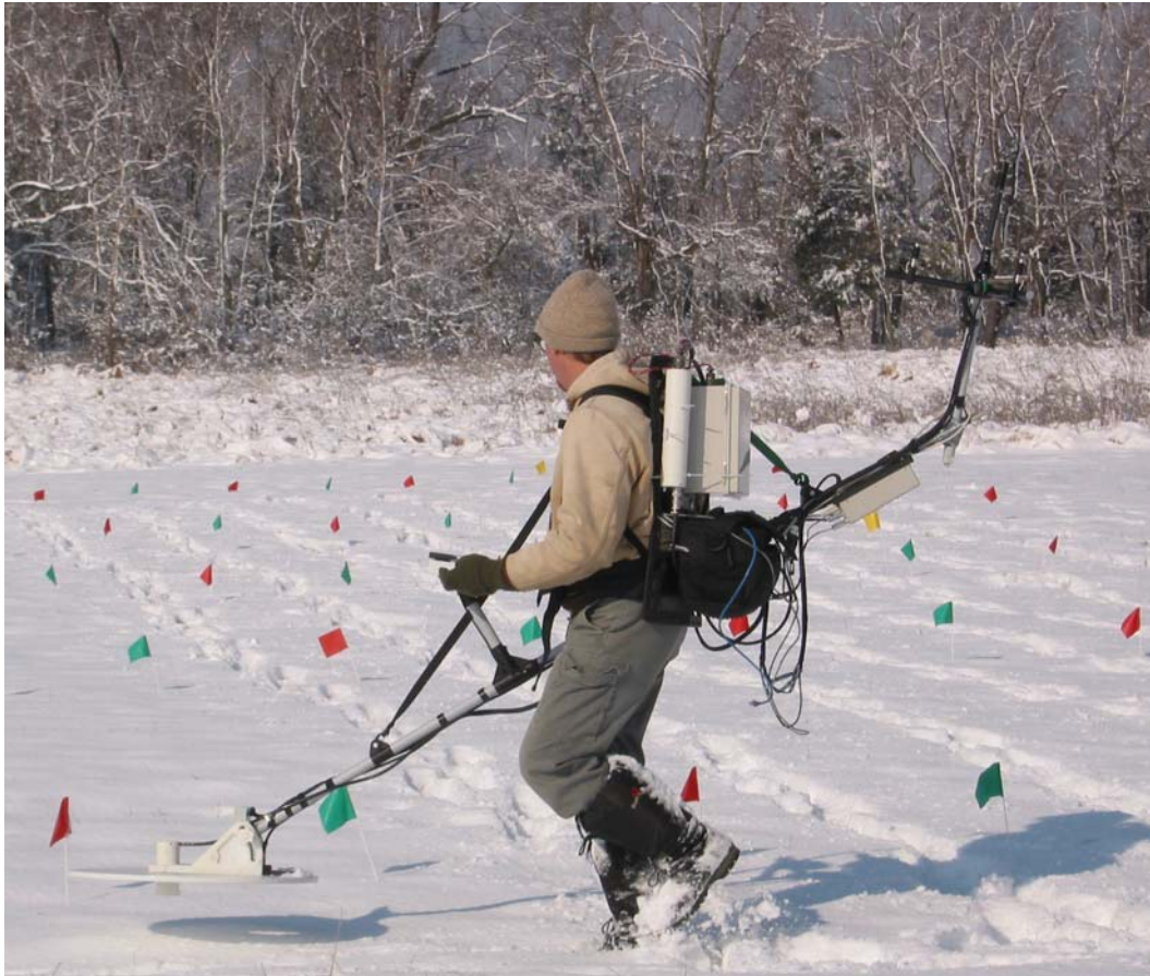
Figure 13. Dual-sensor system deployed in a hand-held configuration at Blossom Point UXO Test Site, MD.
