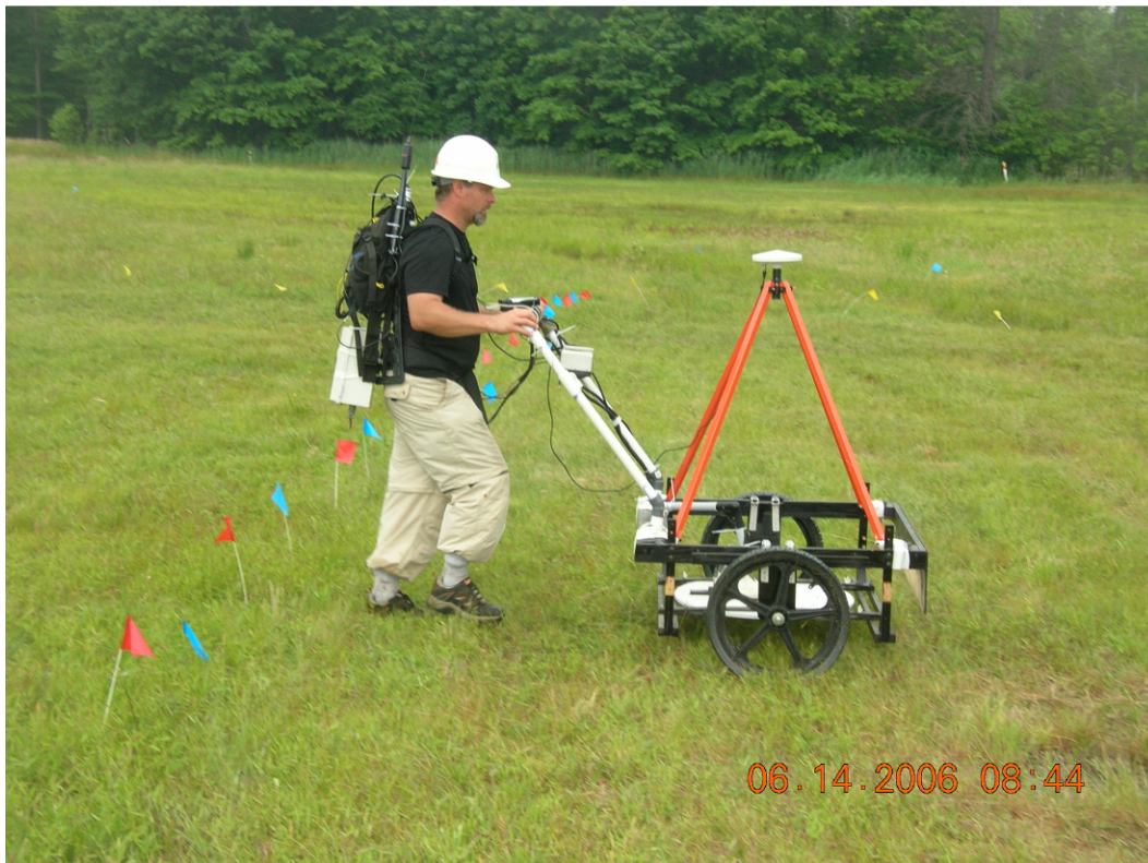
Figure 23. Dual-sensor system reconfigured into a push cart configuration.
