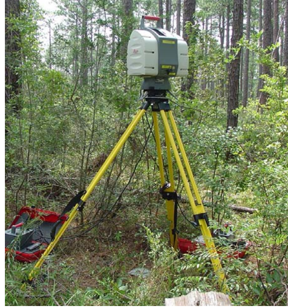
Figure 9. The Leica HDS3000 (ground-based) 3D LiDAR unit utilized for this study.
