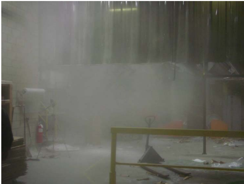
Figure 5: Precision cutting room during blow-down cleaning with compressed air, Claremont Flock Corporation, 2005.
