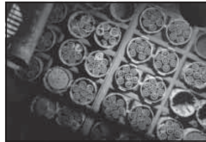
Spent nuclear fuel elements in one of the K-Basins.
