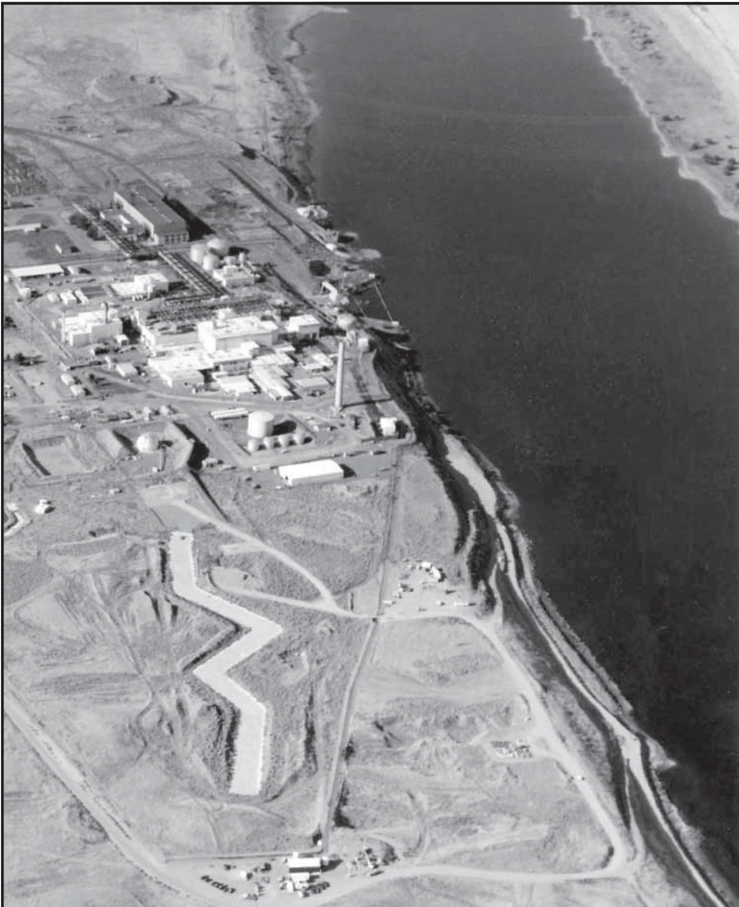
Some Hanford facilities — such as N Reactor above — are located very close to the Columbia River. The zig-zag trench at the bottom of the photo was a liquid waste disposal trench. Another trench is just out of view, farther to the left. The soil and groundwater between the trench and the river is heavily contaminated.
