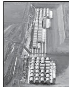
Submarine and cruiser reactor compartments in a trench at Hanford.
