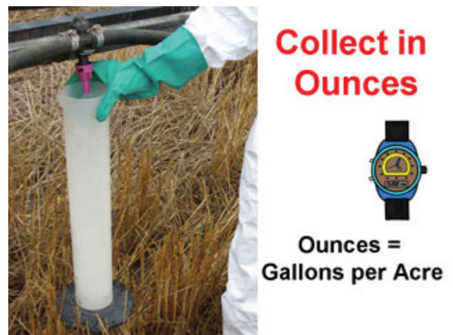
Figure 2. In stationary position and proper boom pressure, measure the output over the same time period to made the run. The number of ounces collected is equal to the gallons per acre.
