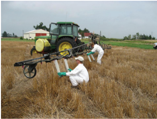
Figure 3. Check the discharge from each nozzle across the boom.
