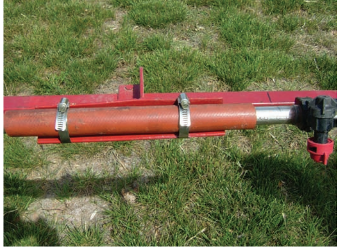
Figure 4. The bracket to hold the wet boom. The rubber hose protects the boom and the stainless steel hose clamps hold the wet boom in place.
