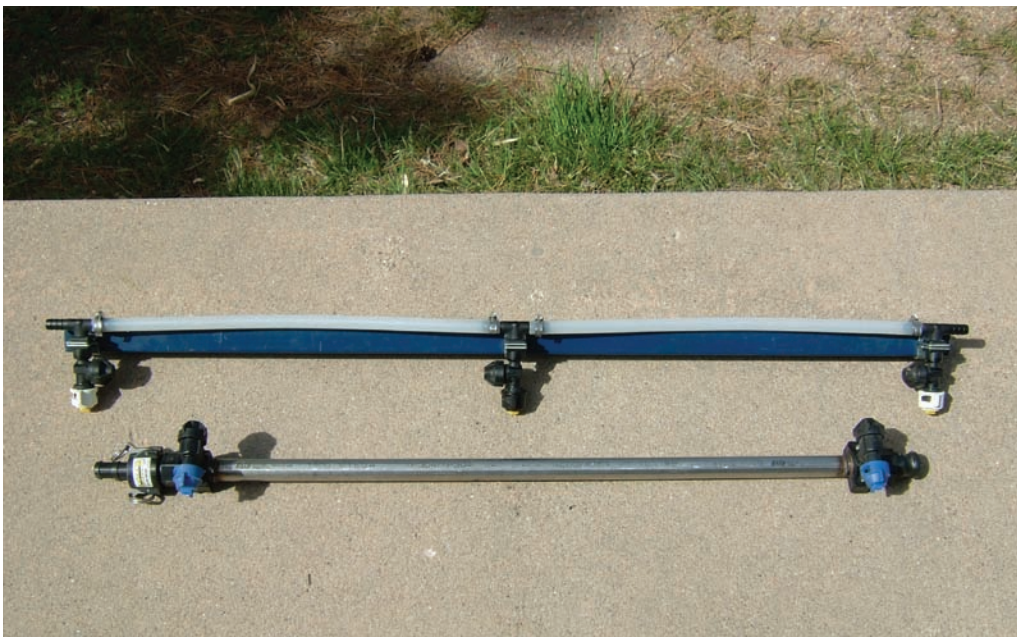
Figure 1. Sections of two booms — dry boom on top, wet boom on bottom.
