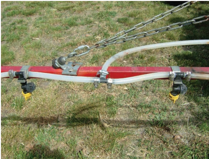
Figure 5. How dry boom is fed — note restriction to flow rate.
