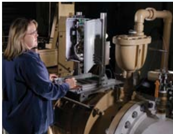
A chemist at Sandia National Laboratories observes a new high-tech unattended water sensor, which constantly monitors water for biological pathogens including biotoxins, bacteria, viruses, and protozoa. Image courtesy of Sandia National Laboratories.
