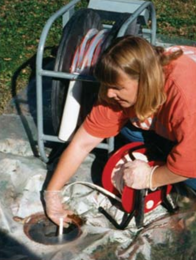
A USGS scientist measures the water level in a monitoring well. The framework for regulating drinking water includes many federal agencies, state regulations, local municipalities, and private organizations. Image courtesy of the USGS.
