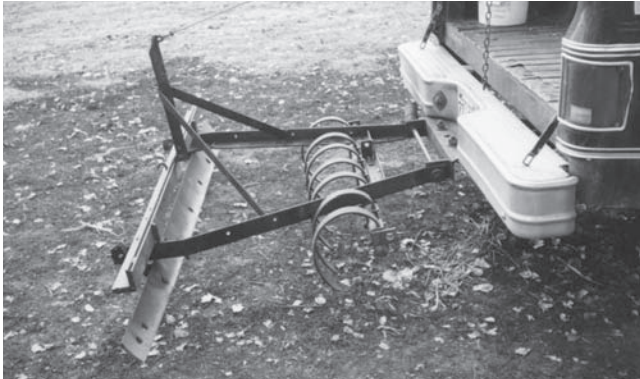
Figure 5. A scraper blade or harrow operation following the burrow builder operation is one technique used to evaluate control.
